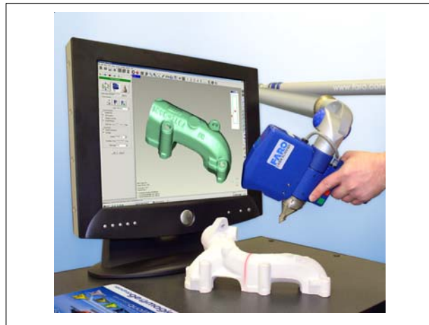
Figure 2. Laser scanners are often mounted on coordinate measuring machines or, in this case, on articulated arms, such as the Faro ScanArm shown here.
